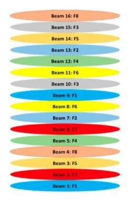
Each satellite has 16 user beams, arranged in a "venetian blind" pattern.
