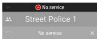
When the PMR Status Bar is **grey**, there is either **no TETRA network coverage** or an **error related to group communication**. The reason for the error is displayed in the header of the status bar.
