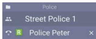
When the PMR Status Bar is **light blue**, the device is **receiving**. A group call is ongoing and the user is listening to the possible group communication, but is not pressing the PTT.
