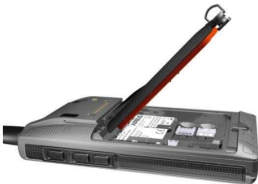
3. Insert the contact end of the battery.
